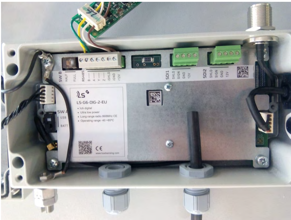
Figure 44: View of the inside of the digital datalogger.
