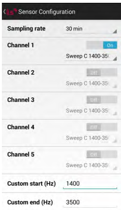
Figure 7: Sensor configuration options of LS-G6-VW-5ch.
