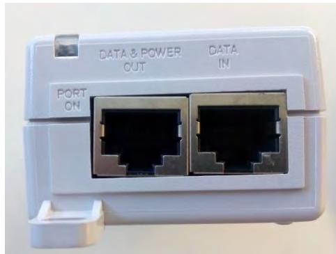
Figure 24: PoE. Left port (Data & Power Out) is for the Power Cable and right port (Data in) is for the Data transmission.
