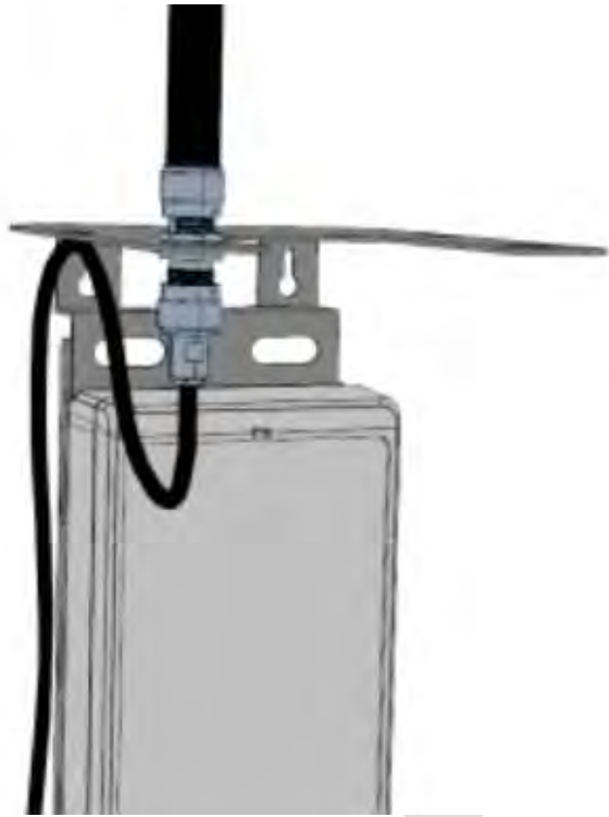
Figure 20: Gateway's antenna mounting.
