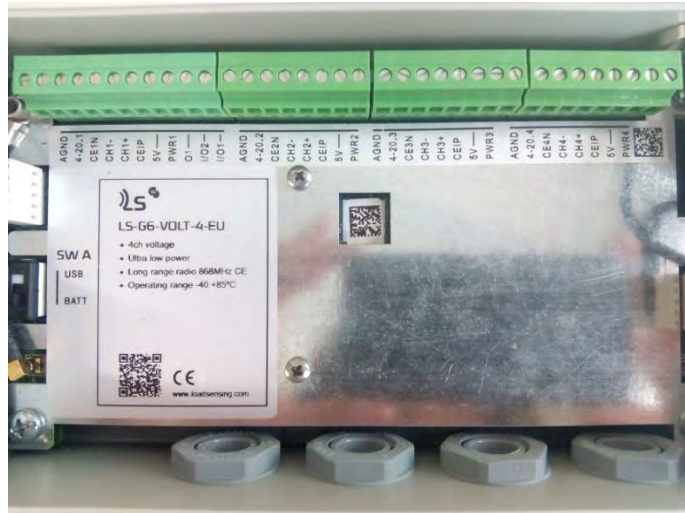
Figure 45: View of the LS-G6-ANALOG datalogger internally where the four channels can be identified.
