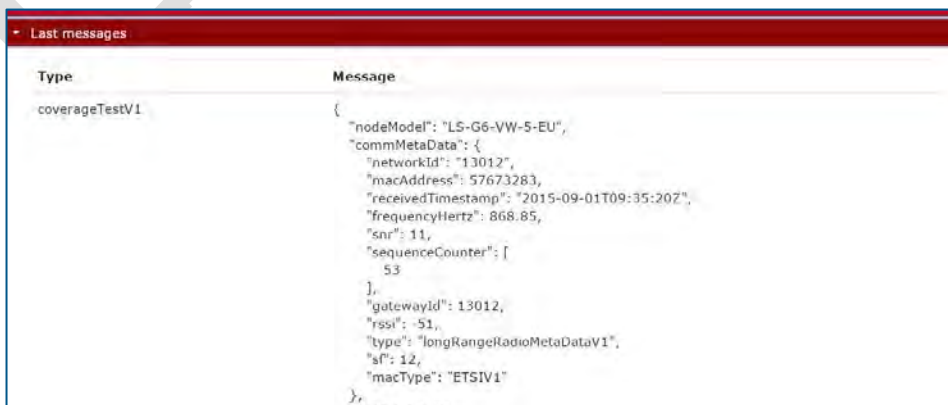
Figure 42: View of last messages received by the gateway, displayed in API format.
