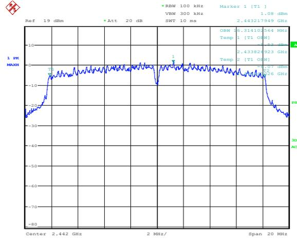
**Figure 8.5-5:** 99% bandwidth on mid channel
