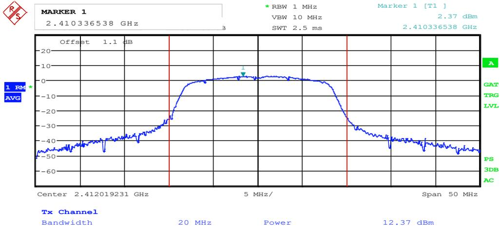
Figure 8.6-1: Output power on low channel
