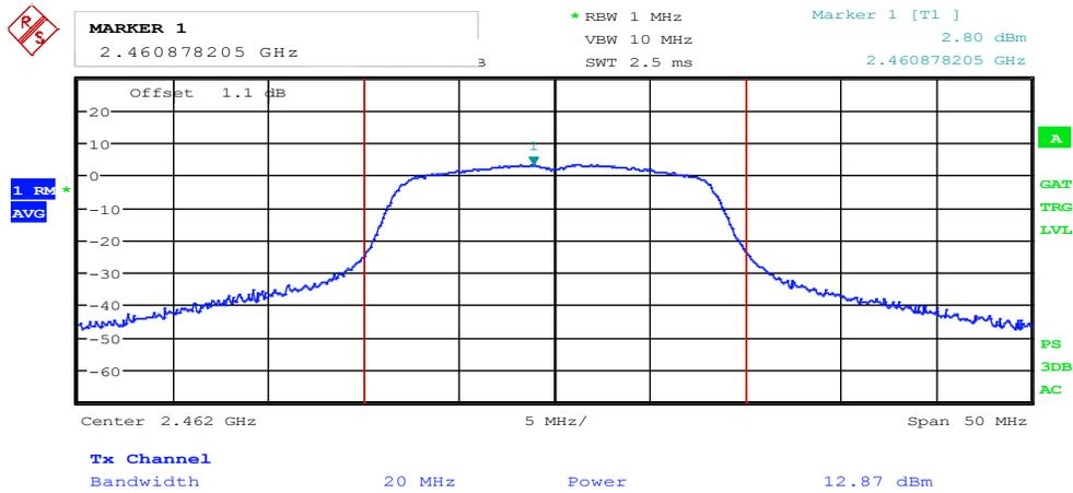
Figure 8.6-2: Output power on High channel
