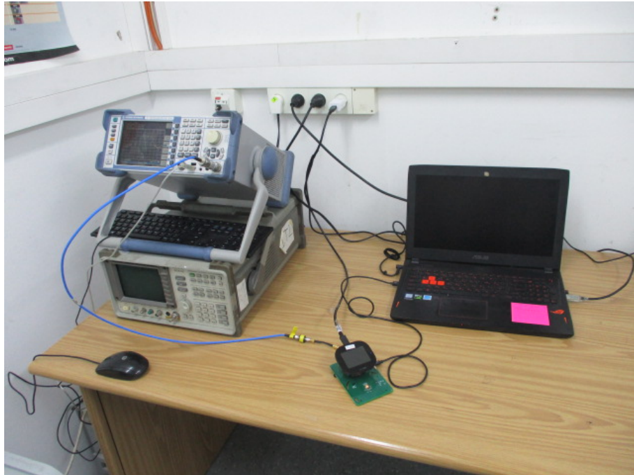
Figure 4. Conducted Emission Test
