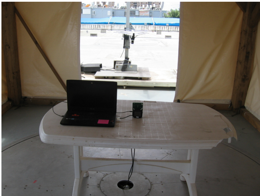
Figure 7. Radiated Emission Test, 200.0-1000.0MHz
