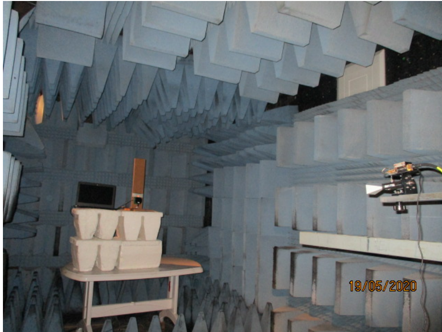
Figure 10. Radiated Emission Test, 26.5-40.0GHz
