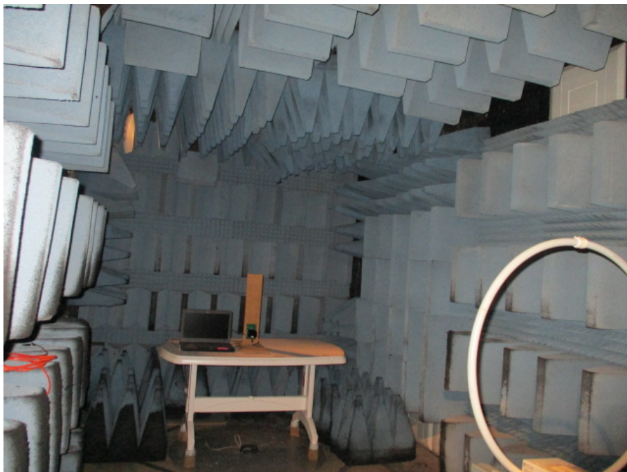
Figure 5. Radiated Emission Test, 0.009-30.0MHz
