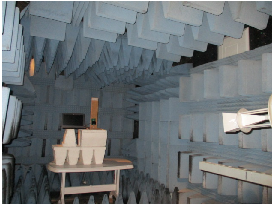
Figure 9. Radiated Emission Test, 18-26.5GHz
