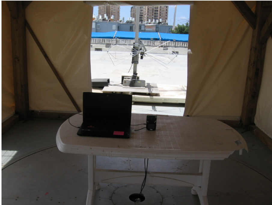
Figure 6. Radiated Emission Test, 30.0-200.0MHz
