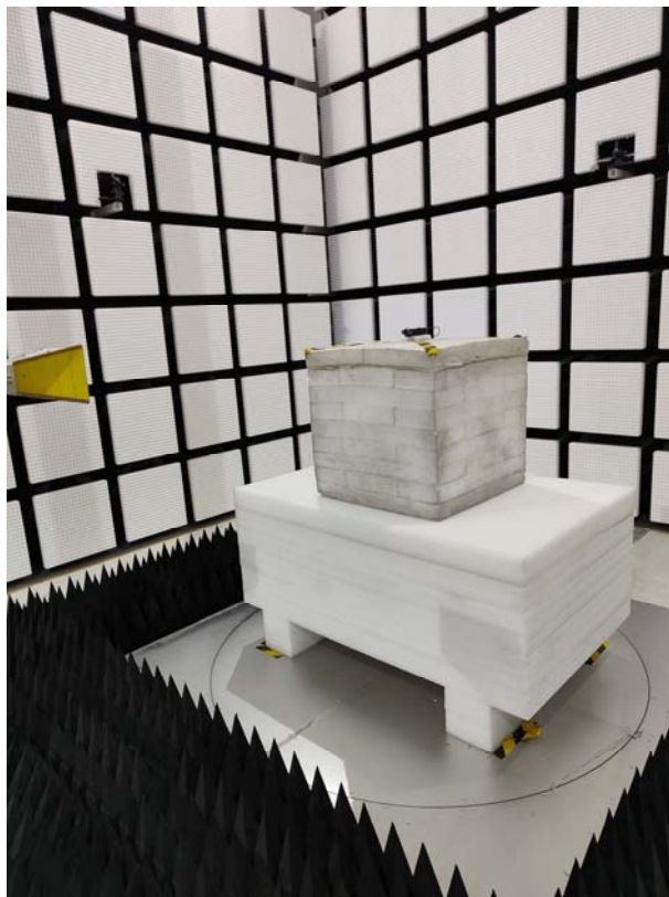
Radiated Emission Above 1GHz View
