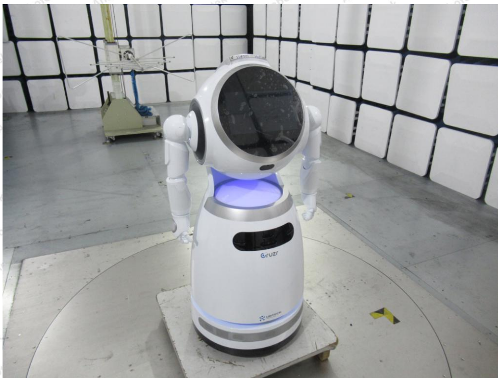
Photo of Radiation Emission Test
