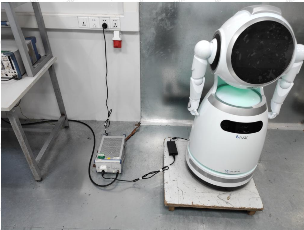
Photo of Power Line Conducted Emission Test
