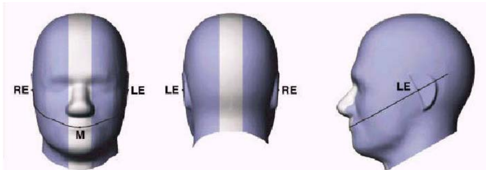
Fig. 9.1 Illustration for Cheek Position
