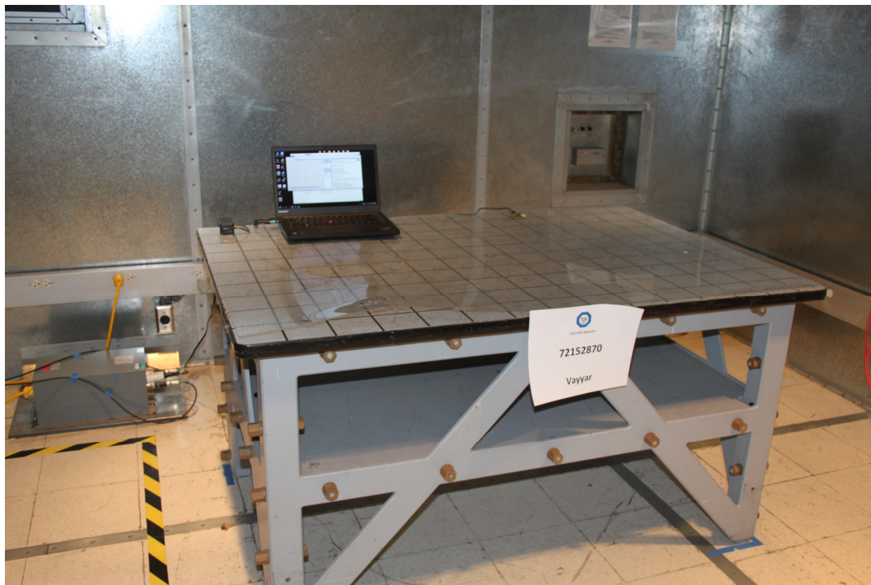
AC Conducted Emissions Test Setup
