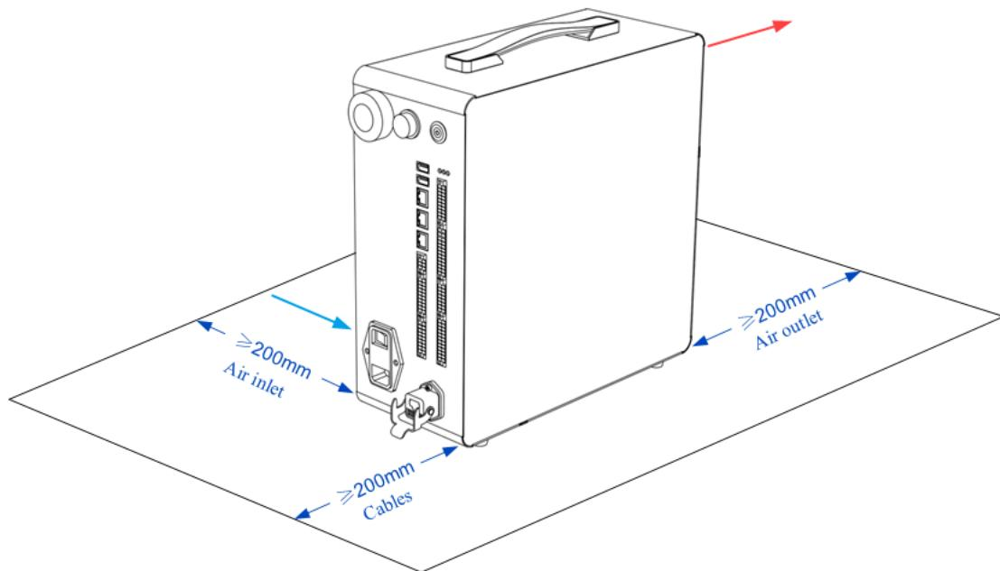
Figure 7.3 Vertical-type installation
