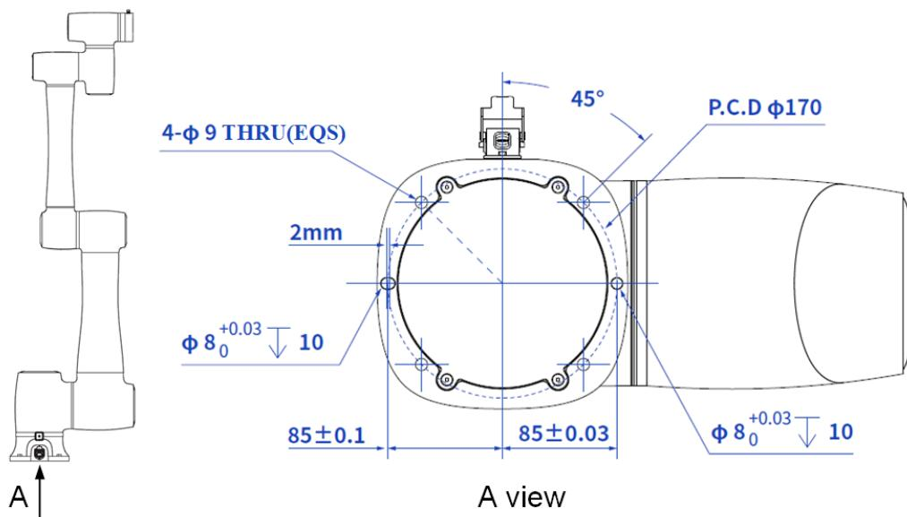
Figure 5.18 CR12A base installation dimensions
