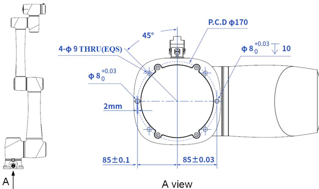
Figure 5.14 CR10A base installation dimensions
