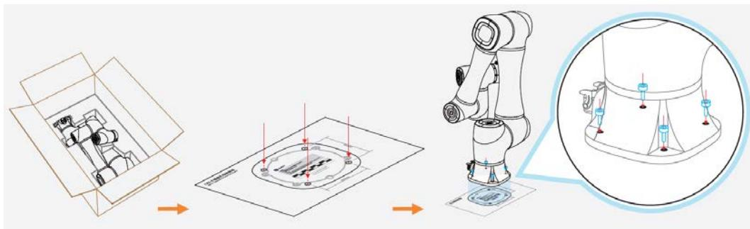
Figure 7.2 CR A robot installation posture
