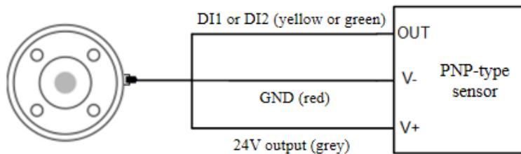
Figure 6.19 Tool DI connected to PNP-type sensor
