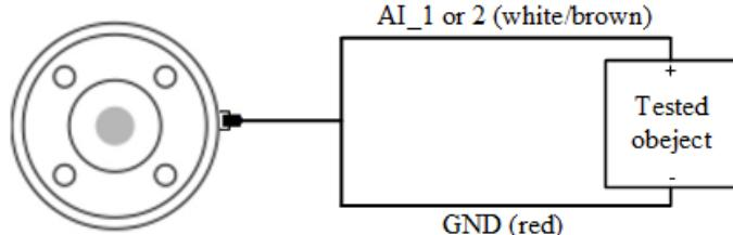
Figure 6.21 Tool AI wiring
