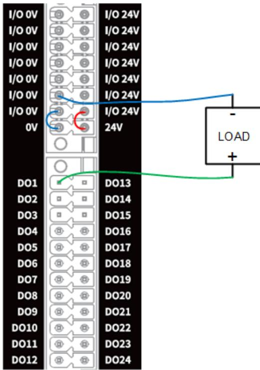
Figure 6.8 PNP-type DO connected to external load
