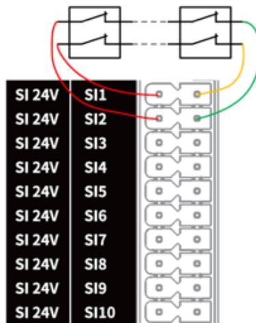
Figure 6.15 SI connected to multiple emergency stop switches
