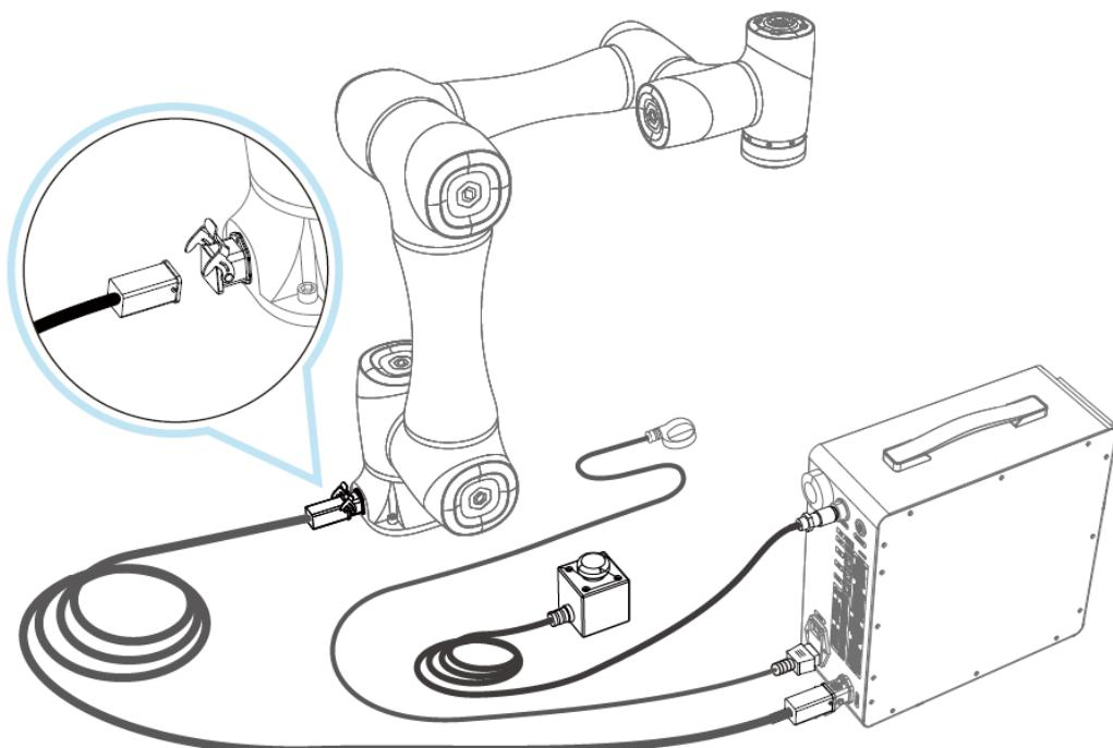
Figure 7.8 Wiring diagram
