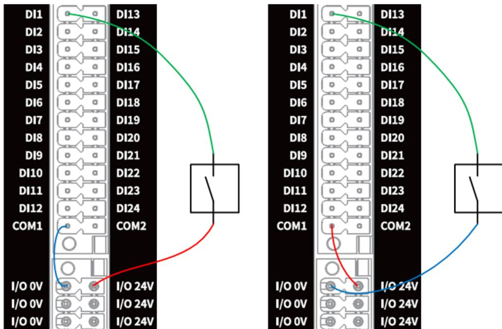
Figure 6.5 DI connected to simple switch
