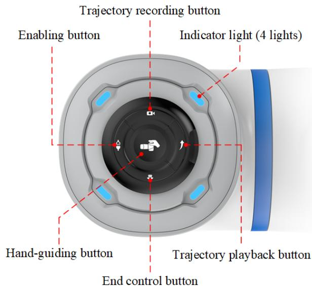
Figure 3.5 End buttons and indicator light (except CR20A)
