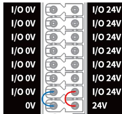
Figure 6.3 I/O connected to internal power supply
