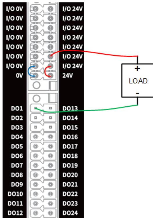
Figure 6.9 NPN-type DO connected to external load
