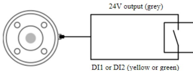
Figure 6.18 Tool DI connected to simple switch
