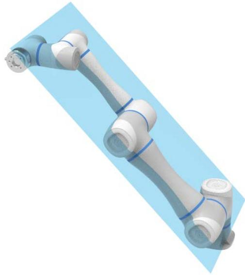
Figure 4.6 Elbow singularity
