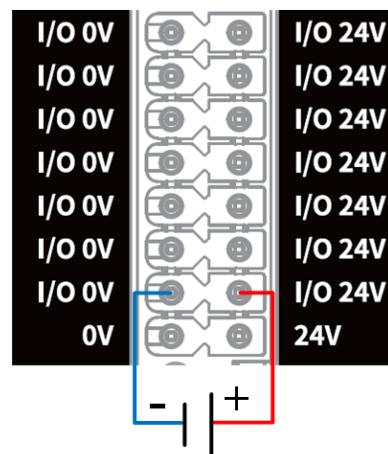
Figure 6.4 I/O connected to external power source
