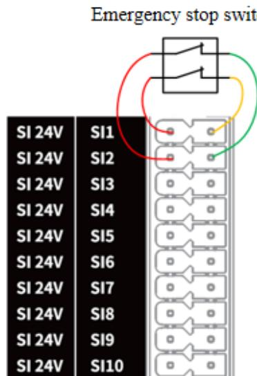
Figure 6.14 SI connected to one emergency stop switch
