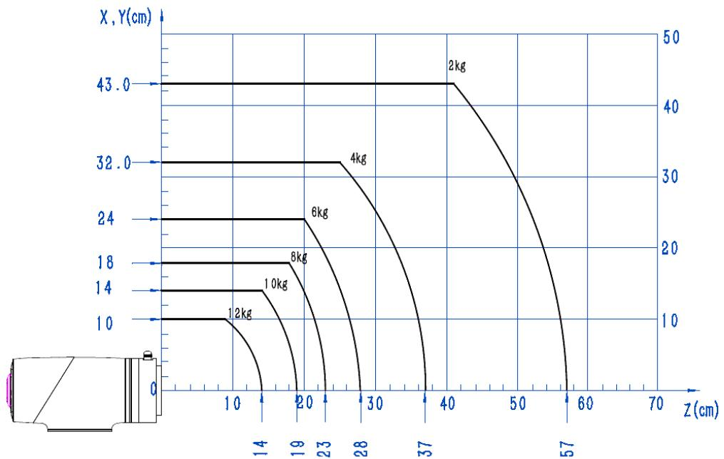
Figure 5.20 CR12A load curve
