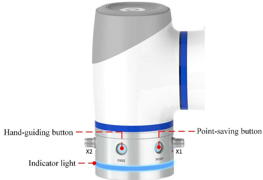
Figure 3.6 End buttons and indicator light (CR20A)
