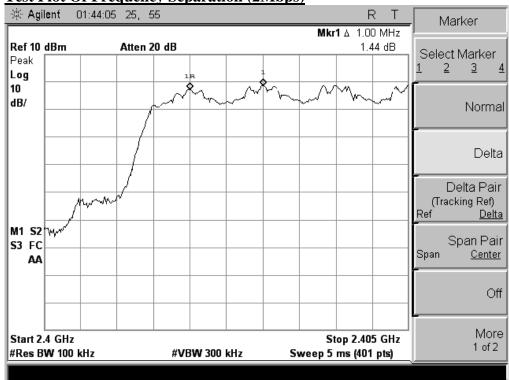
**Test Plot Of Frequency Separation (3Mbps)**
