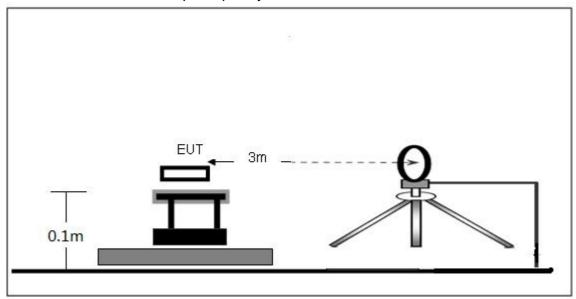
(B) Radiated Emission Test-Up Frequency 30MHz~1GHz
