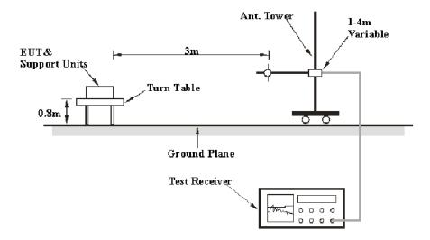
The radiated emission tests were performed in the 3-meter chamber test site, using the setup accordance with the ANSI C63.10-2013. The specification used was the FCC 15.209 limits.
