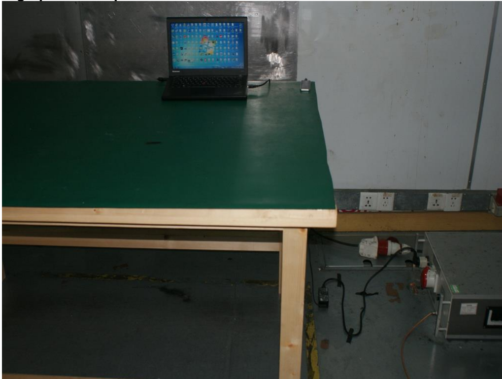
Photograph 6: Set-up for Radiated Emission
