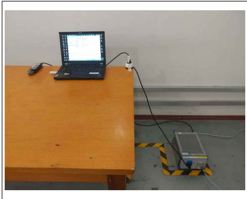
Photo of AC Power line emission Test
