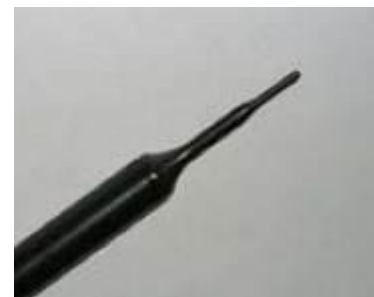
Picture C.2 Near-field Probe
