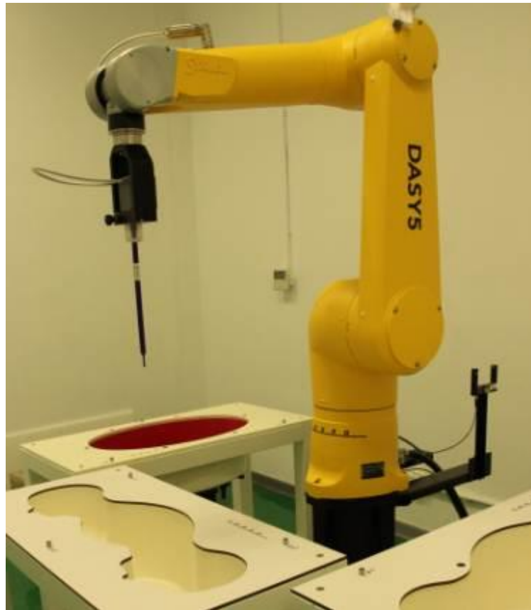
Picture D.6 DSY5 system Set-up
