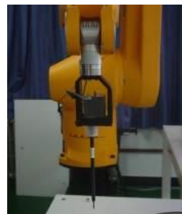
Picture C.2 Near-field Probe
