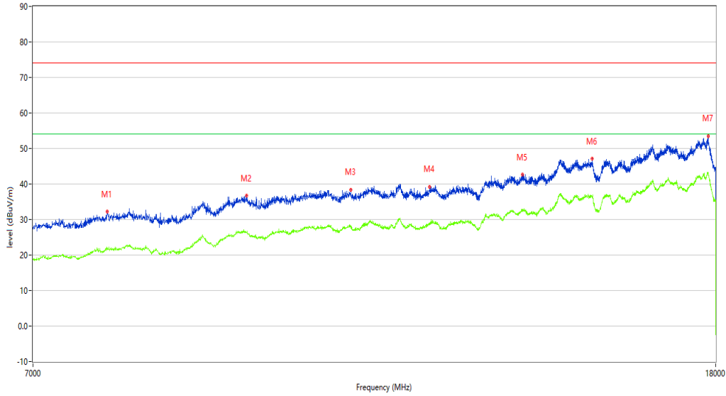
REmission Test case_FCC_Part 15C_FCC 15.247_7GHz-18GHz
