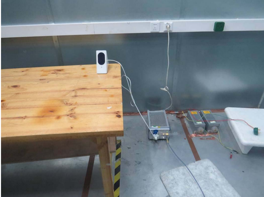
Picture 3 Conducted Emission Test Setup
