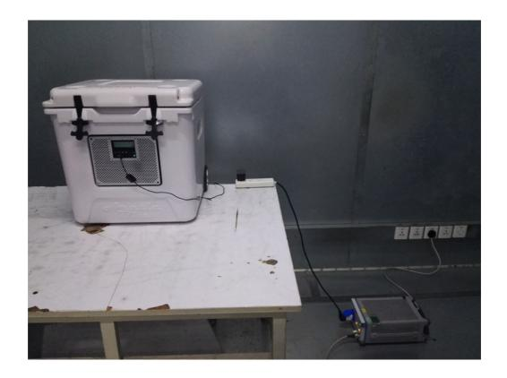
**Radiated Emission Test**
