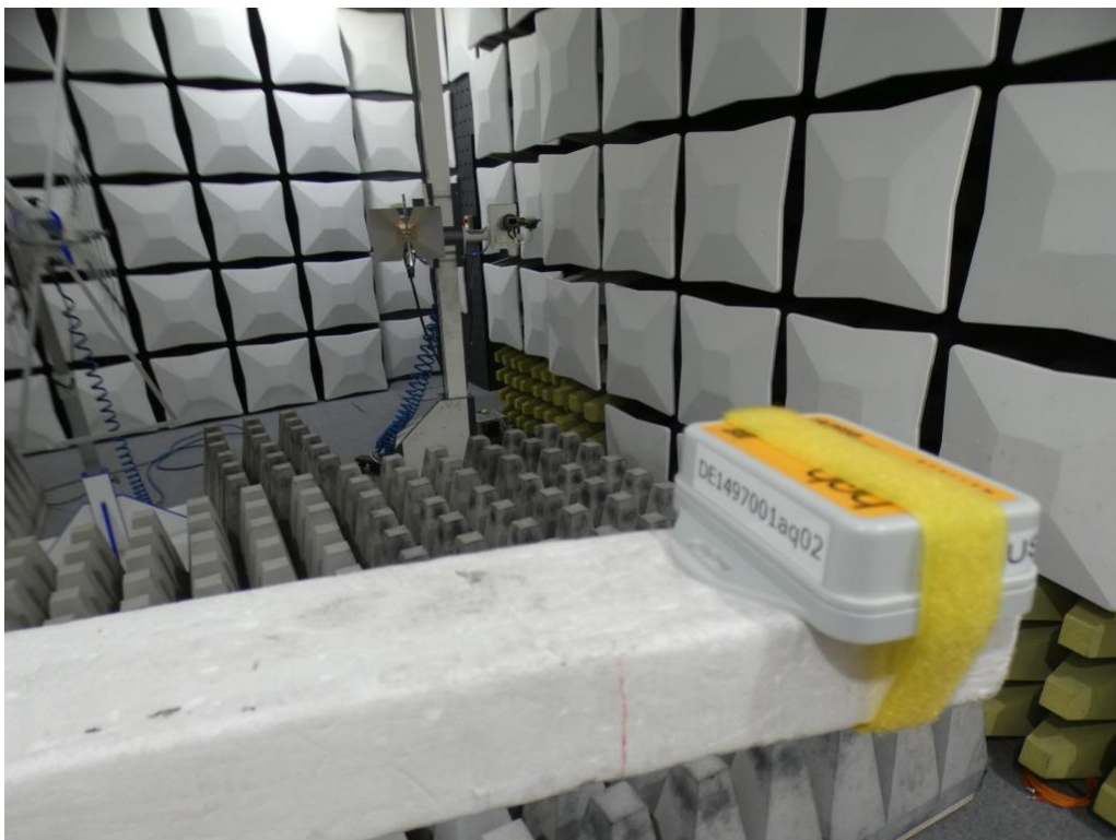
Photo 6: Test setup for radiated measurements, detailed view (Fully anechoic chamber 1 – 10 GHz; FCC Part 15.247; ANSI C63.10)
