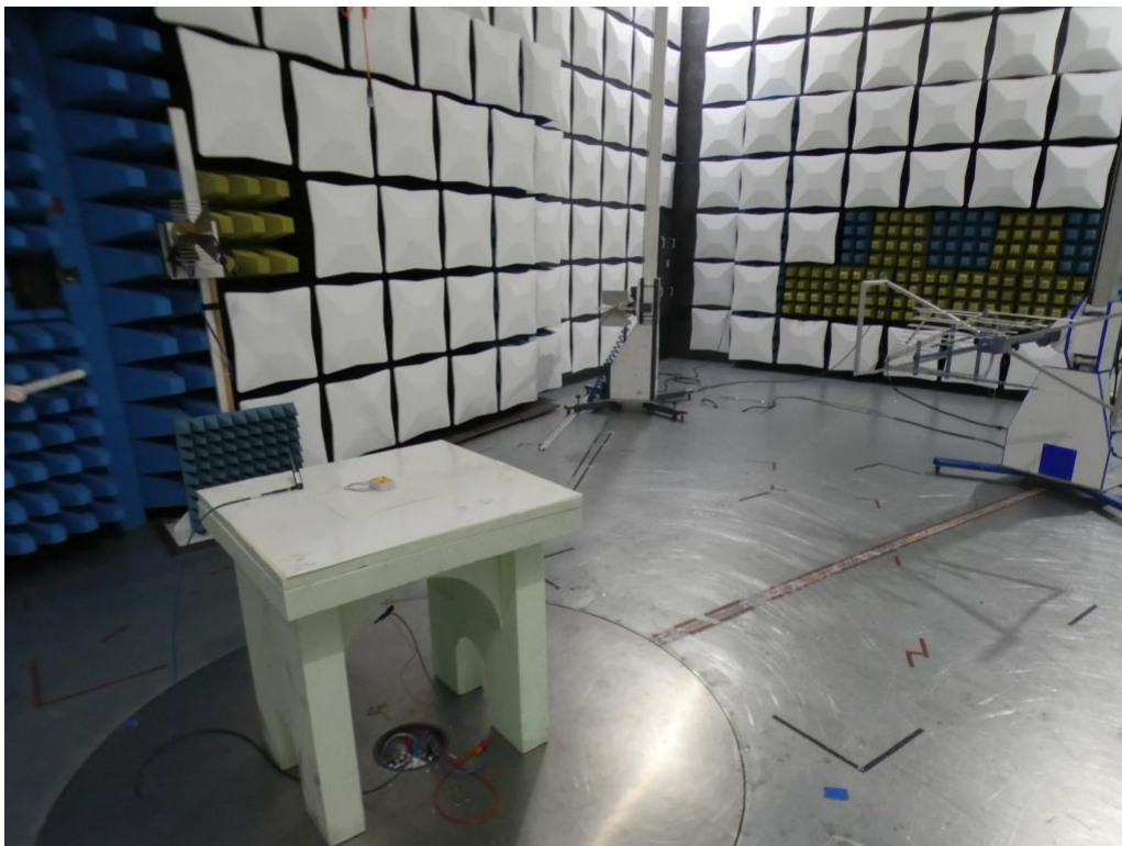
Photo 2: Test setup for radiated measurements (semi-anechoic chamber 30 MHz – 1 GHz; FCC Part 15.247, ANSI C63.10)
