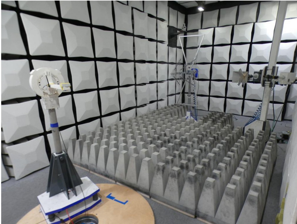
Photo 5: Test setup for radiated measurements (Fully anechoic chamber 1 – 10 GHz; FCC Part 15.247; ANSI C63.10)
