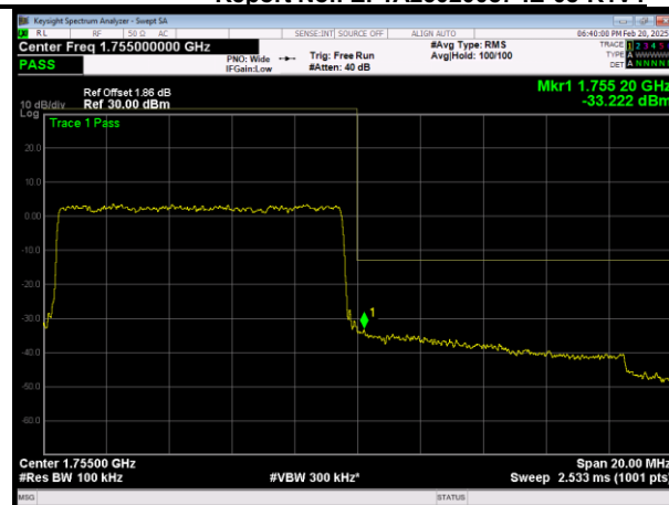
HLTE Band4 QPSK BW=10MHz Channel=20350 RB Size=50 Position=#0
