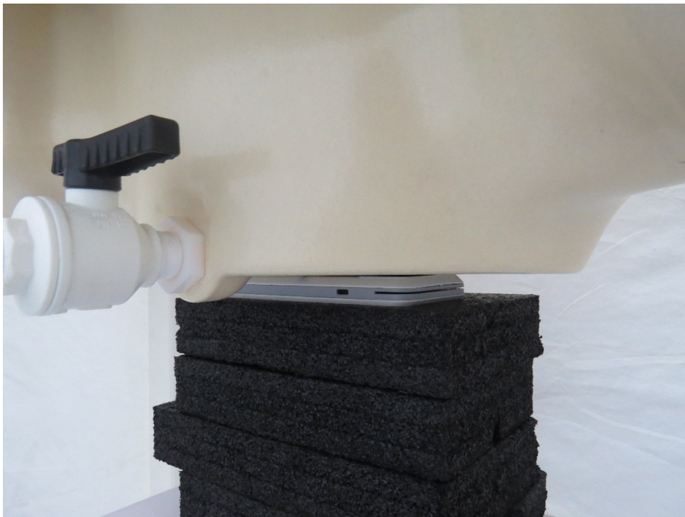
Picture 10: Back Side, the distance from EUT to the bottom of the Phantom is 0mm
