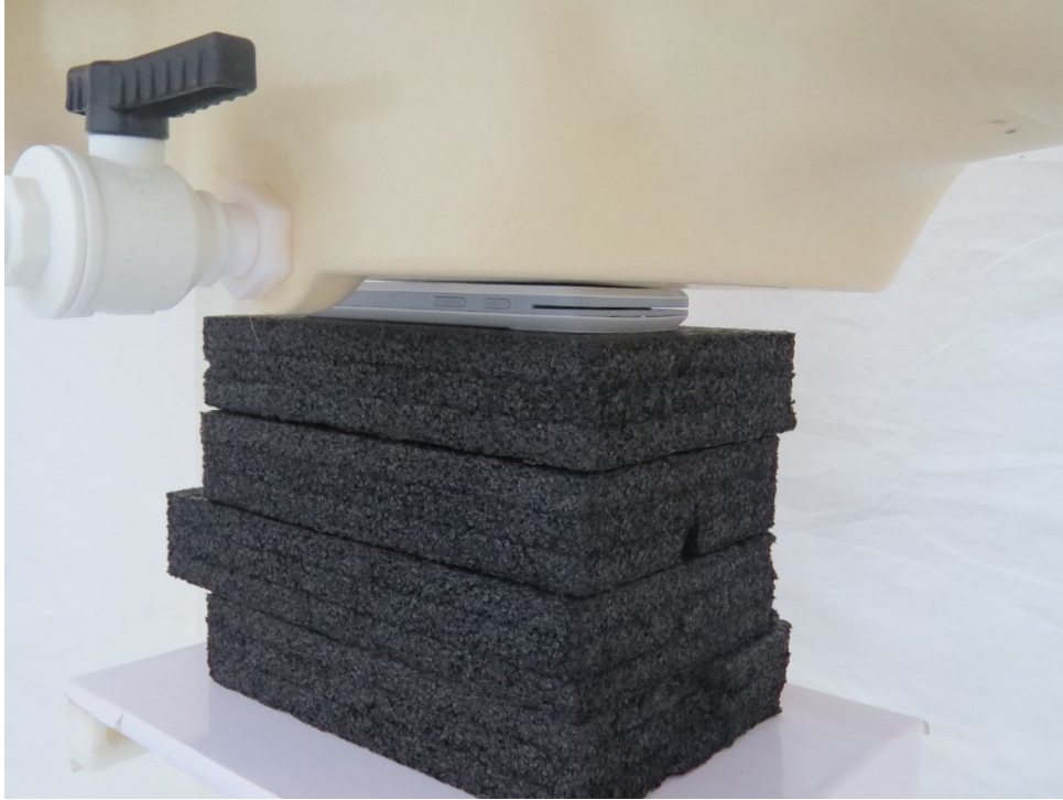
Picture 11: Front Side, the distance from EUT to the bottom of the Phantom is 0mm
