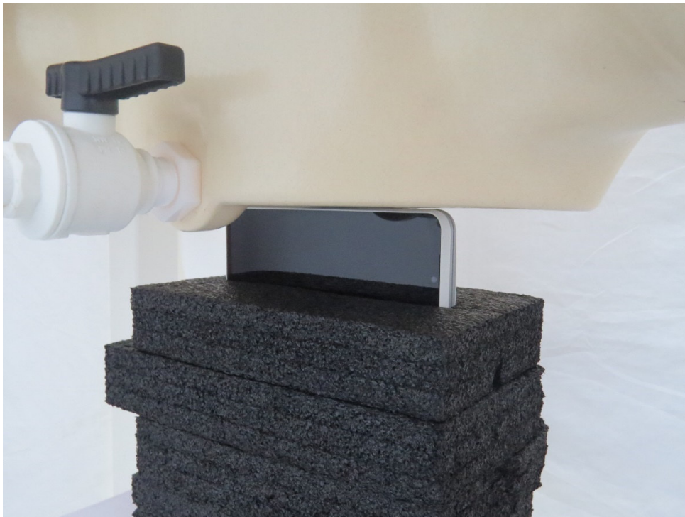
Picture 12: Left Edge, the distance from EUT to the bottom of the Phantom is 0mm
