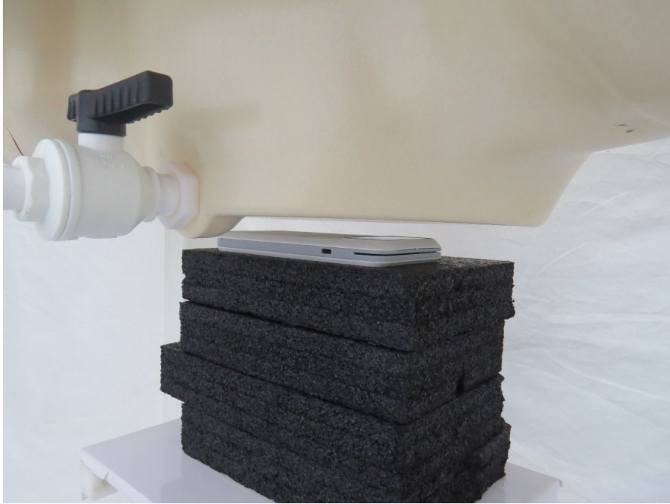
Picture 5: Back Side, the distance from EUT to the bottom of the Phantom is 10mm
