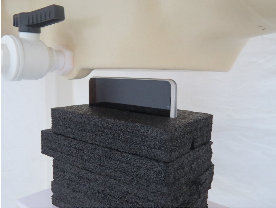
Picture 7: Left Edge, the distance from EUT to the bottom of the Phantom is 10mm
