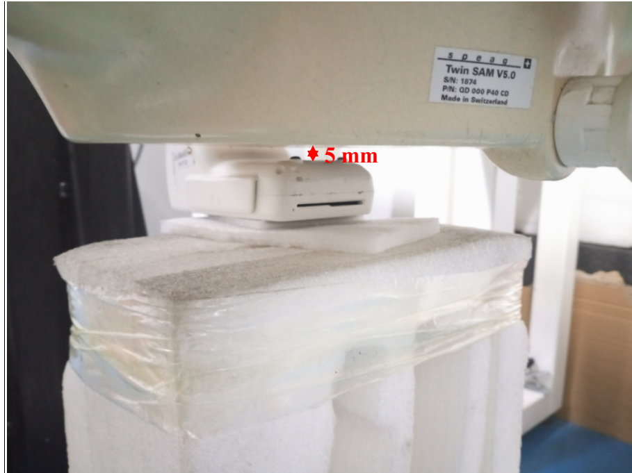
Body Back (WWAN) Setup Photo(5mm)
