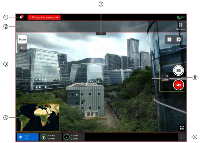
Fig 6-1 Main Interface of the flight application (Fusion 4T Gimbal and in multi-aircraft frequency matching mode)
