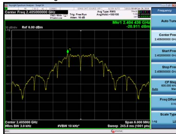
Zigbee, Channel No.: 26
