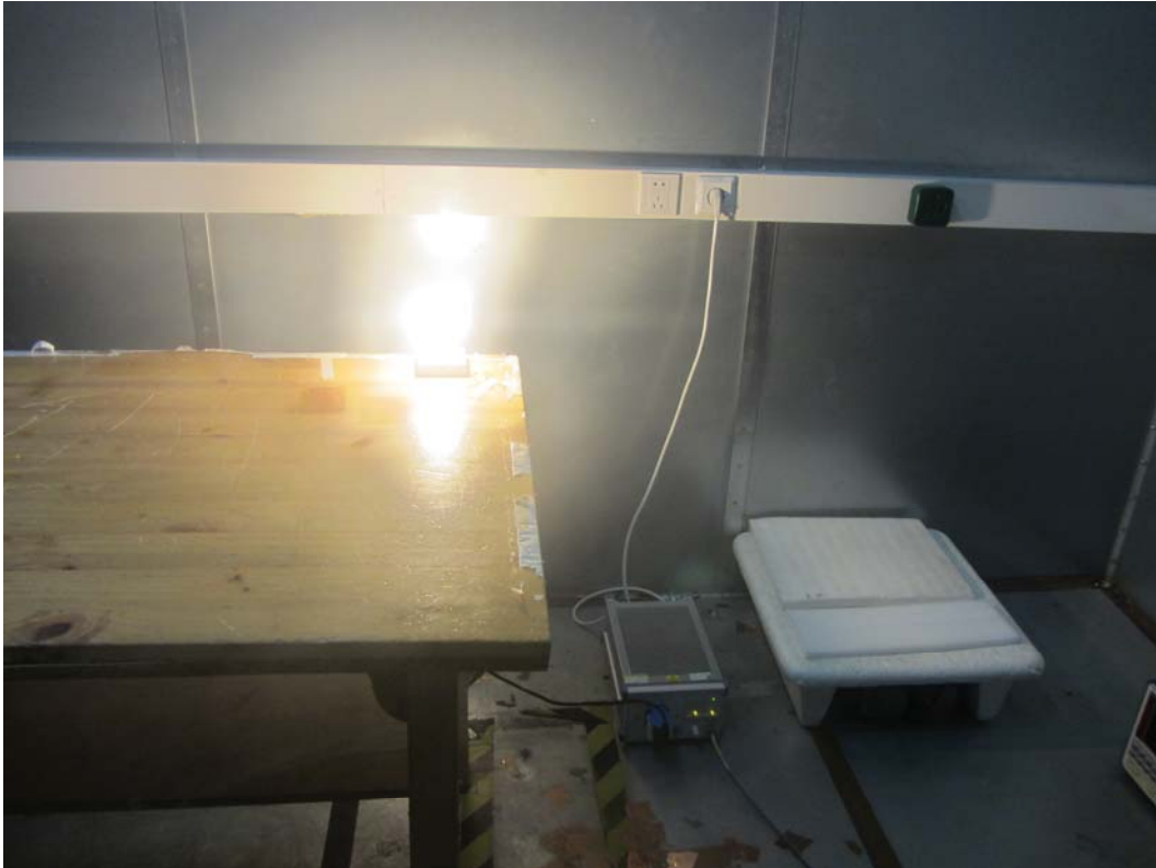
Picture 3 Conducted Emission Test Setup
