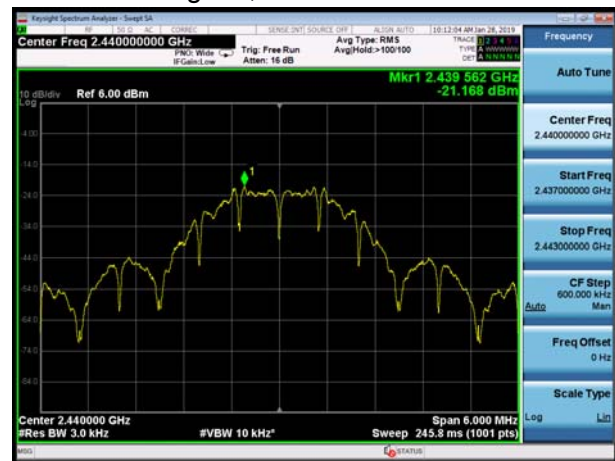
Zigbee, Channel No.: 18
