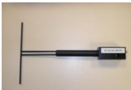
Figure 1 – Satimo COMOSAR Validation Dipole
