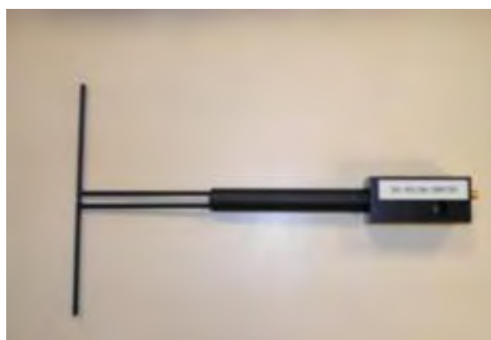
Figure 1 – Satimo COMOSAR Validation Dipole
