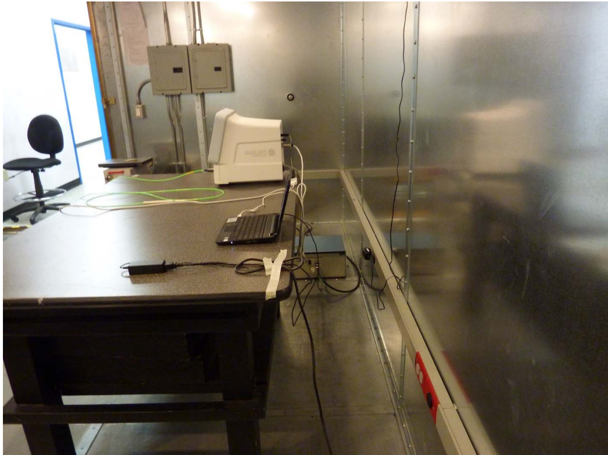
Figure 10 – AC Line Conducted Emissions
