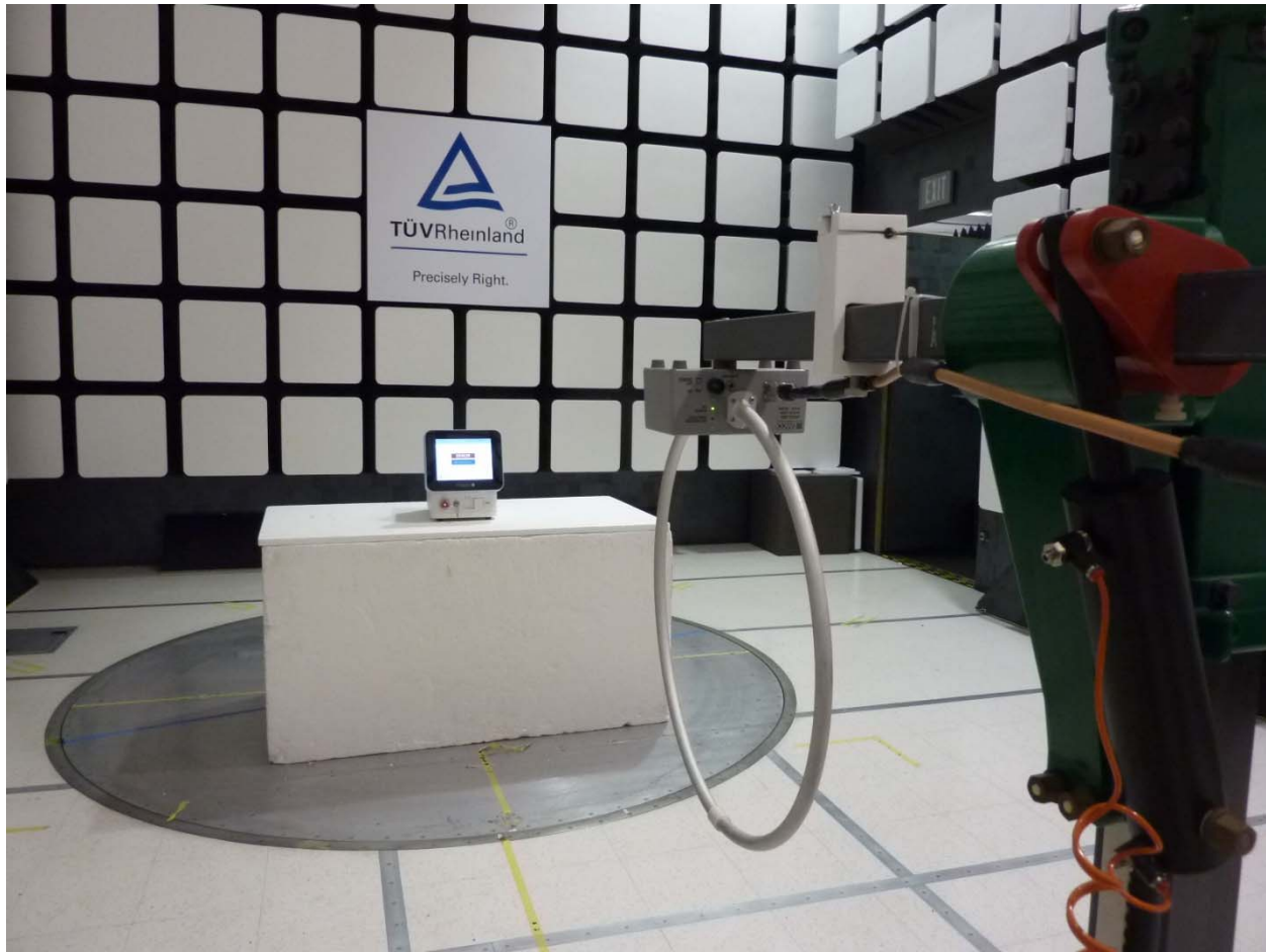
Figure 5 – Radiated Emissions 9 kHz to 30 MHz Antenna Facing EUT 90 Degrees
