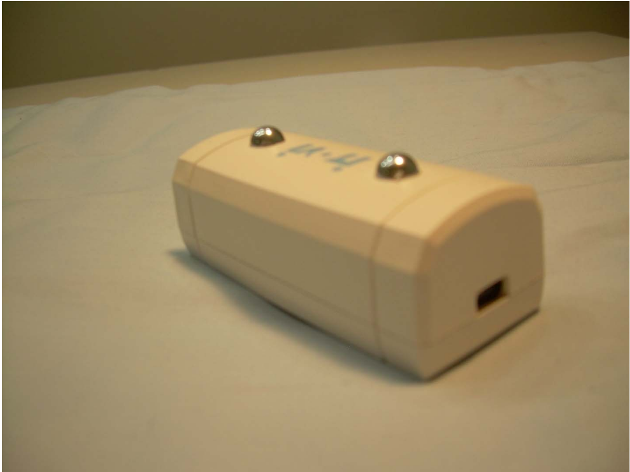
Photograph 9 – View of the Mini USB Port
