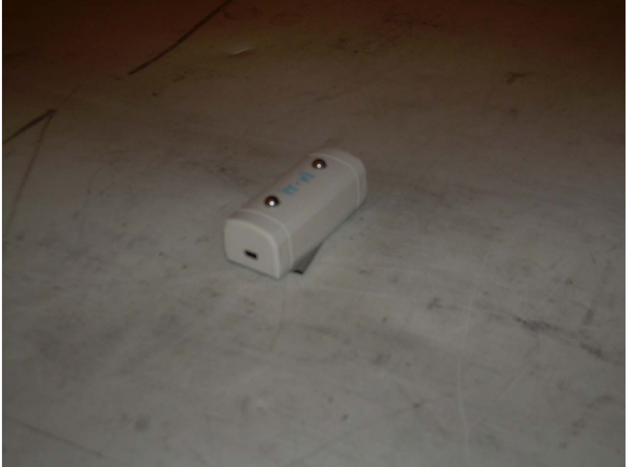
Photograph 3 – View Radiated Emission Configuration – Battery Power, Flat
