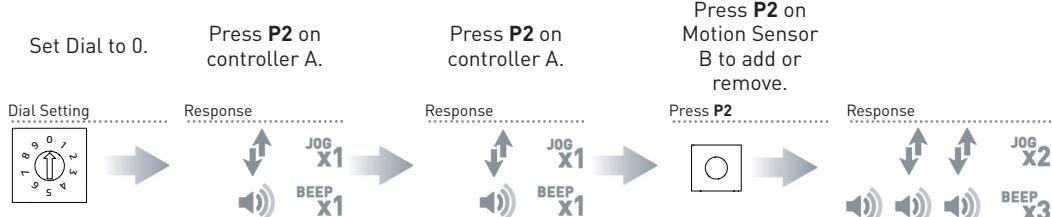
Once paired, confirm Motion sensor is working with motor. To do this, use the Sensor as a Remote.
