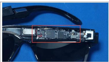
The antenna is Internal antenna.
