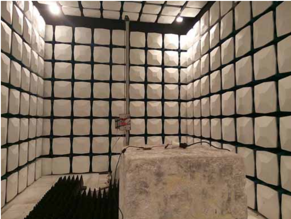
Description: Radiated Emission Test Setup for 1~18GHz
