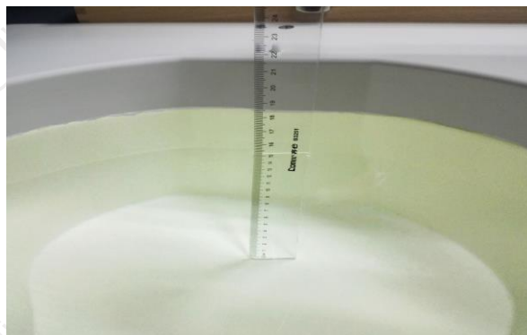
The Body Liquid of 1800MHz (15.2 cm)
