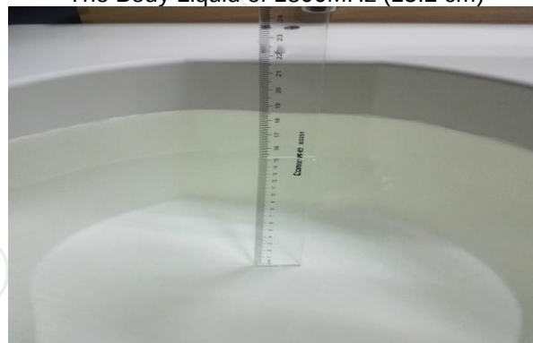
The Body Liquid of 2450MHz (15.3cm)
