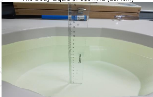
The Body Liquid of 1900MHz (16.4 cm)
