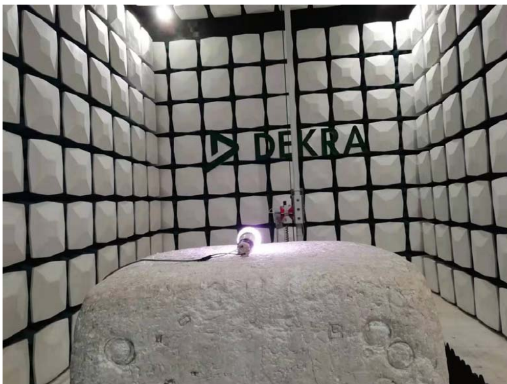
Description: Radiated Emission Test Setup for 1~18GHz
