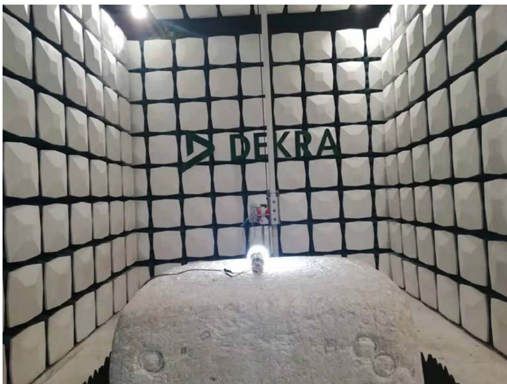
Description: Radiated Emission Test Setup for 1~18GHz
