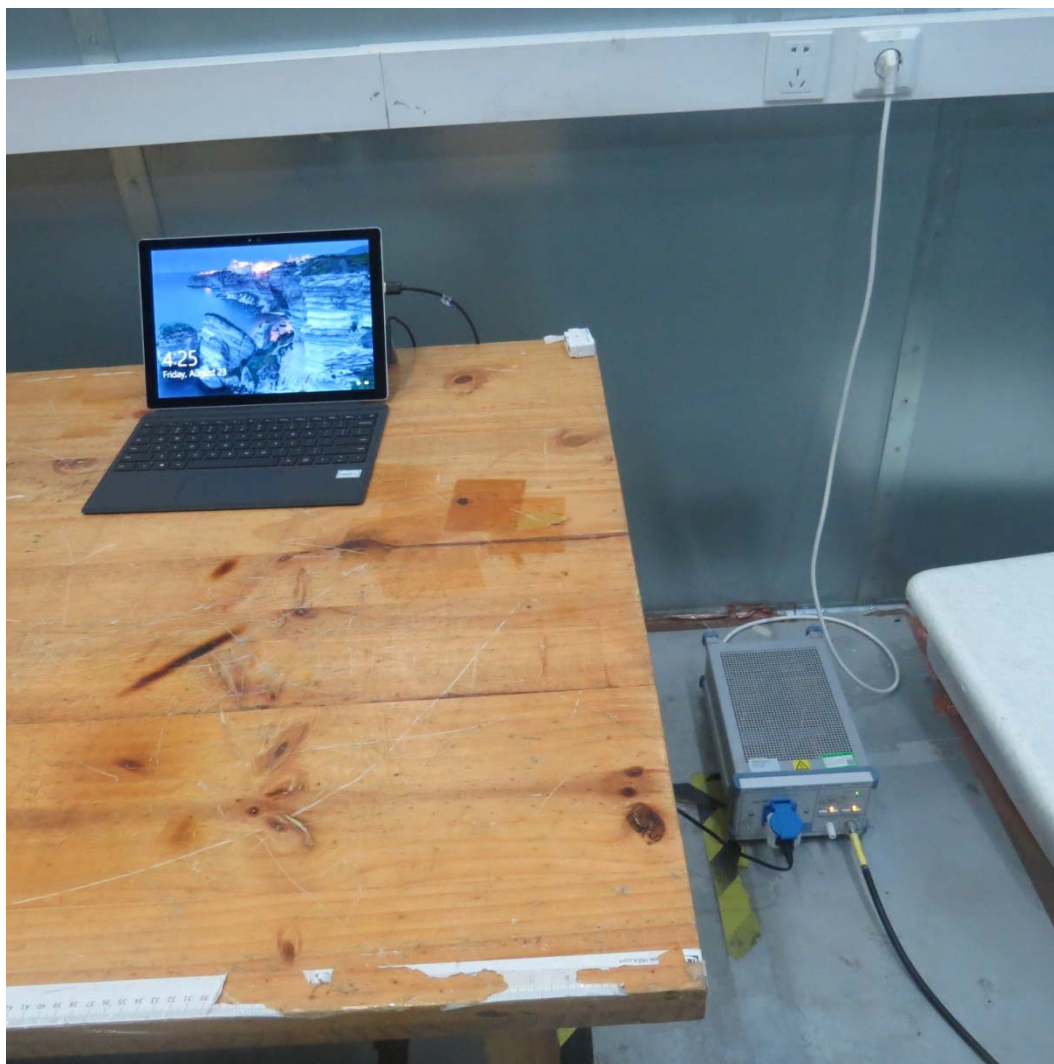
Picture 2 Conducted Emission Test Setup
