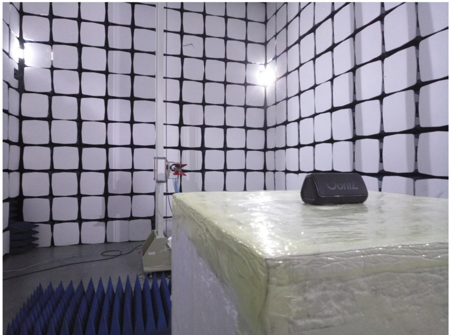
Radiation Emission Test Setup (1GHz to 18GHz)
