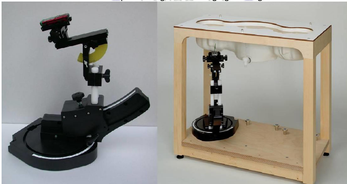
Device holder supplied by SPEAG
