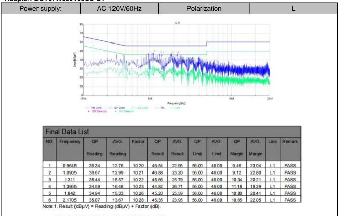
Factor (dB) = Cable loss (dB) + LISN Factor (dB).
