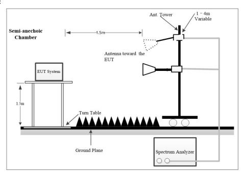
The radiated emission tests were performed in the 3 meters test site, using the setup accordance with the ANSI C63.10-2013. The specification used was the FCC 15.209, and FCC 15.407 limits.
