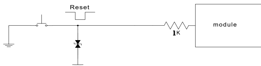
Figure 4.7: Reference design of key reset circuit
