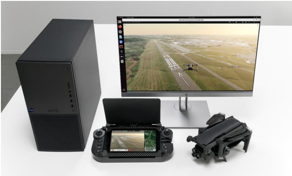
Figure 17: ANAFI UKR and Skycontroller UKR connected to a PC for the simulator
