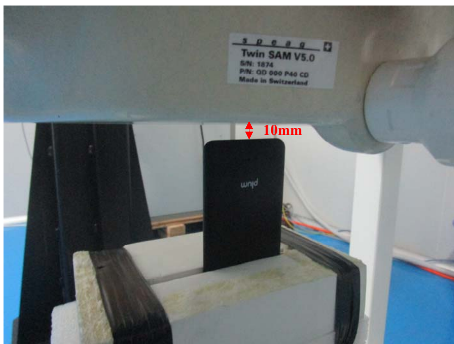
Body-worn Bottom Setup Photo
