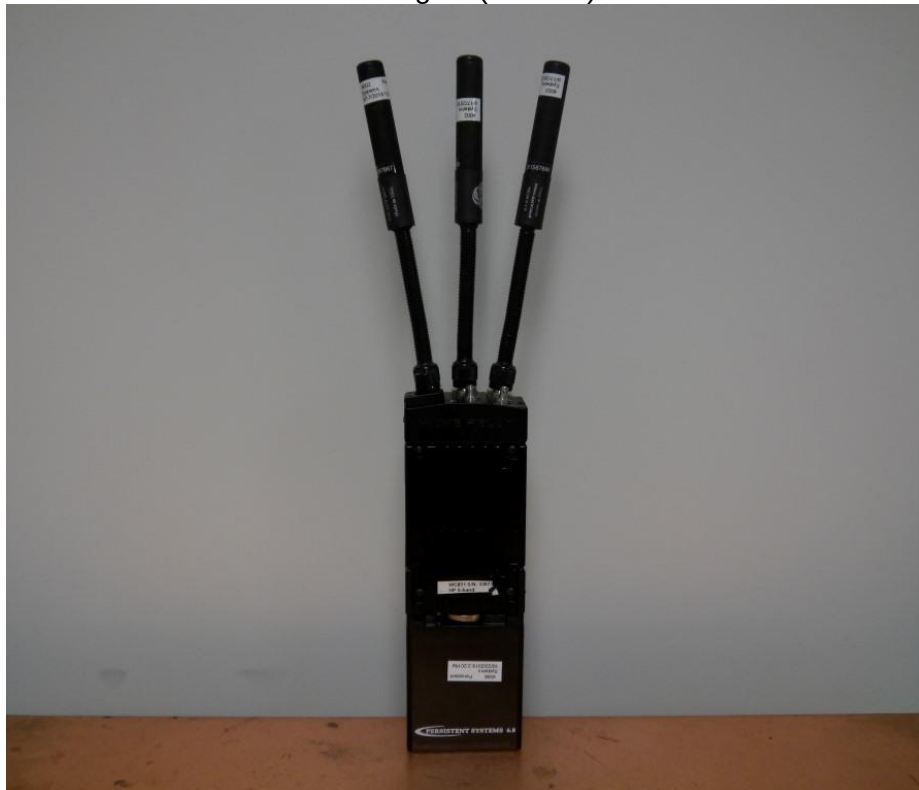
EUT with 3 low-gain (2.15dBi) antennas
