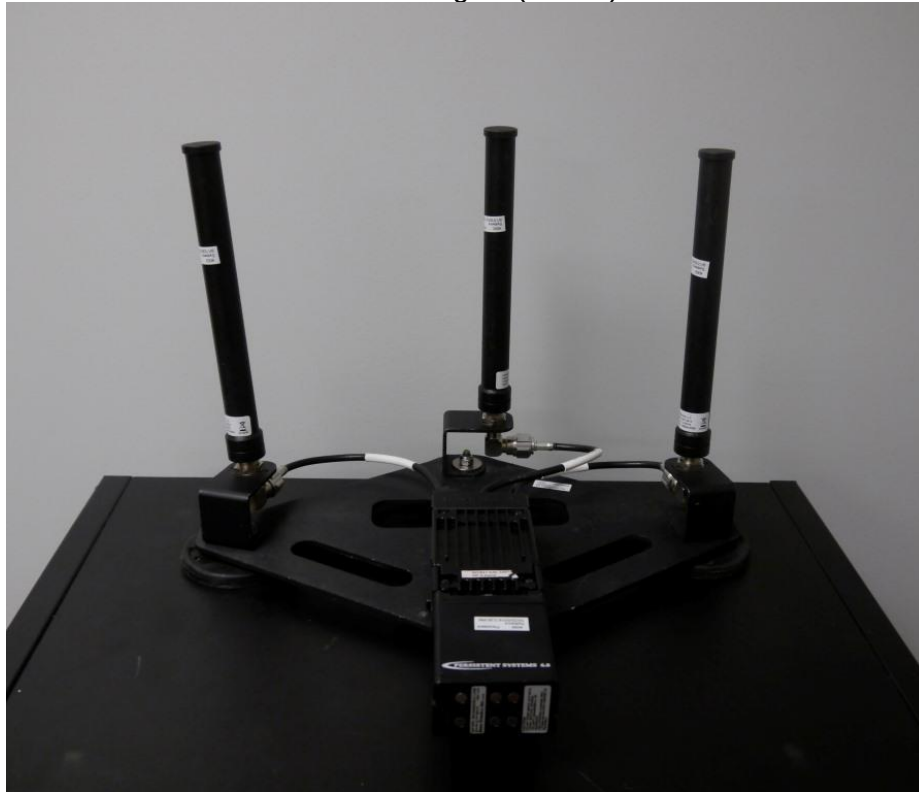
EUT with 3 low-gain (2.15dBi) antennas
