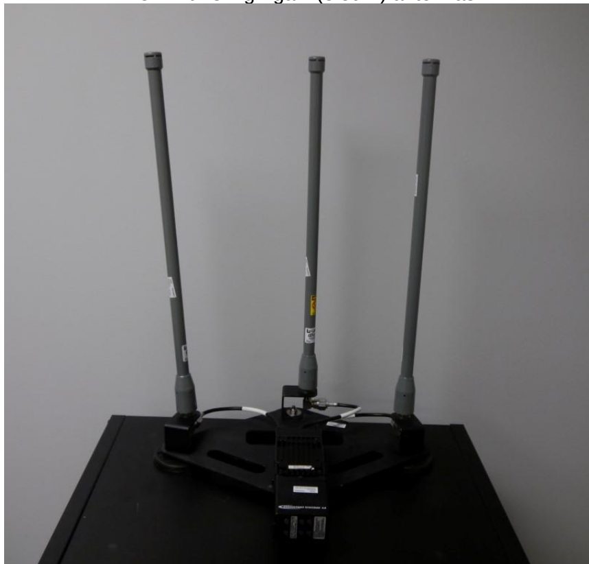
EUT with 3 high-gain (8.5dBi) antennas
