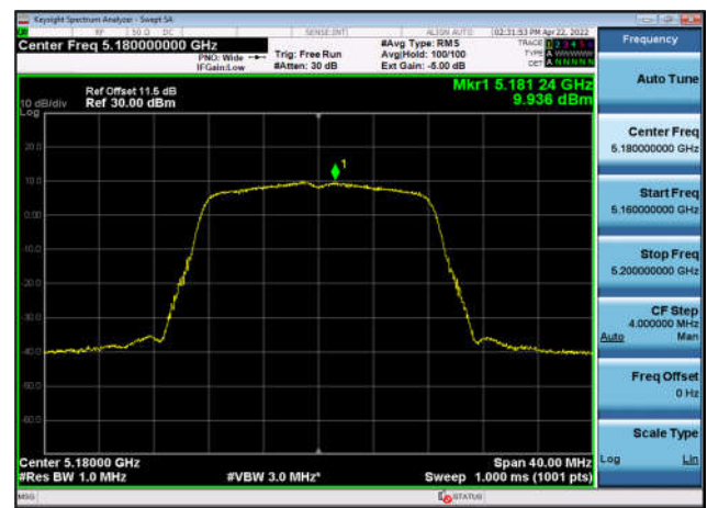
U-NII-1 Power spectral density-802.11 a(20MHz),5180MHz,Ant1
