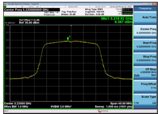
U-NII-1 Power spectral density-802.11 n(40MHz),5190MHz,Ant1
