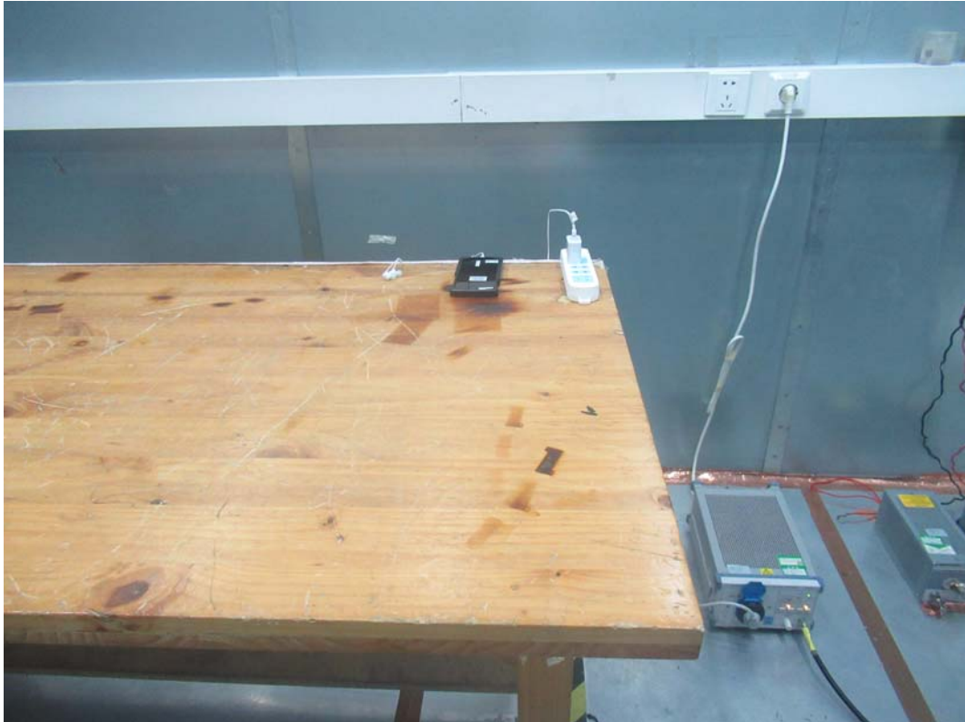
Picture 2 Conducted Emission Test Setup
