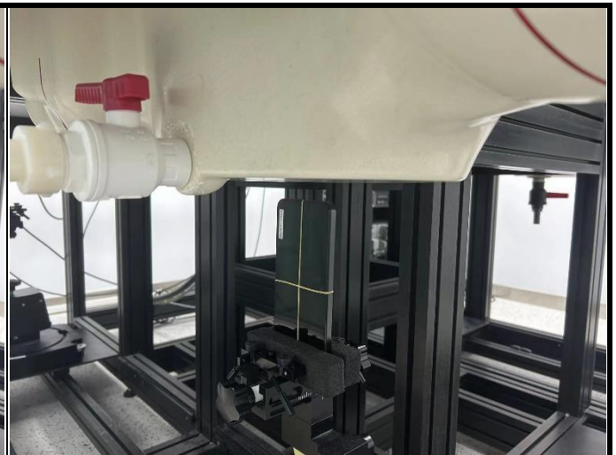
Bottom Side of EUT with 1.9 cm Gap
