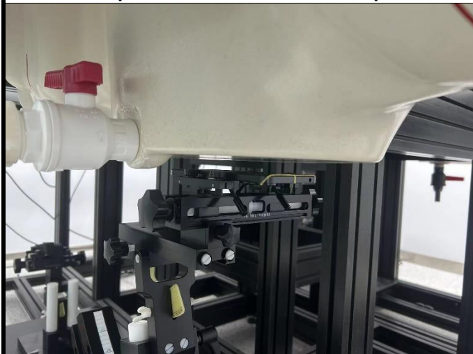
Front Face of EUT with 1.3 cm Gap
