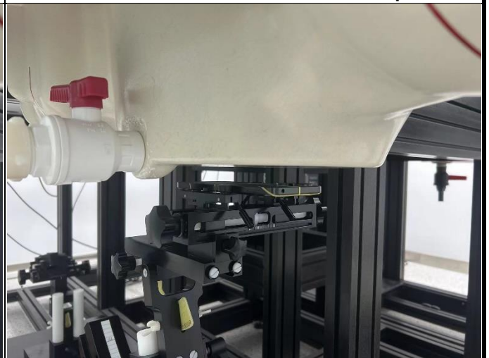
Rear Face of EUT with 1.9 cm Gap
