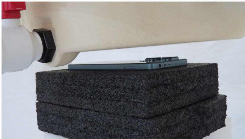
Picture 19: Back Side, the distance from EUT to the bottom of the Phantom is 17mm
