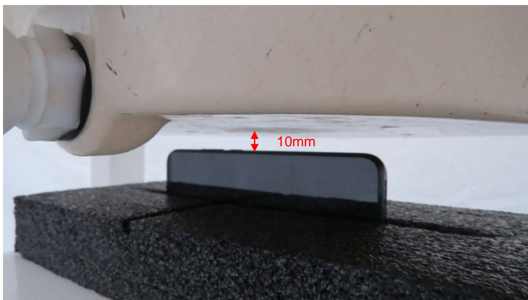
Picture 11: Right Side, the distance from handset to the bottom of the Phantom is 10mm
