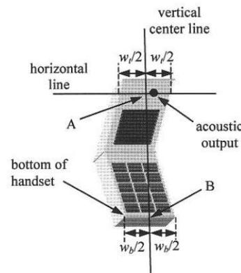
Fig 9.2.2 Handset vertical and horizontal reference lines—“clam-shell case”
