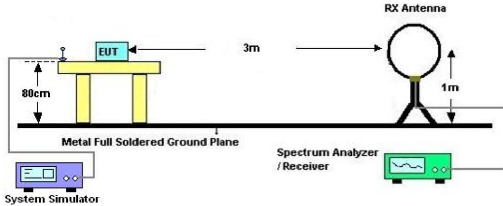
For radiated test from 30MHz to 1GHz
