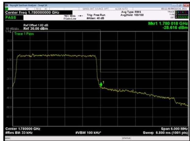
LTE Band 66 QPSK 5MHz CH-High, 1 RB
