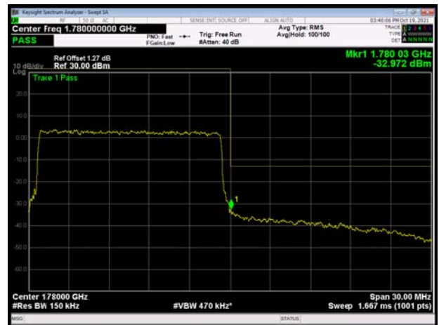
LTE Band 66 64QAM 20MHz CH-High, 1 RB
