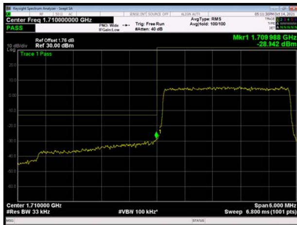
LTE Band 66 QPSK 5MHz CH-Low, 1 RB
