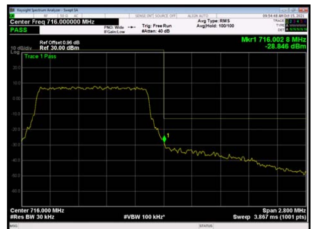
LTE Band 12 64QAM 1.4MHz CH-High, 100%RB
