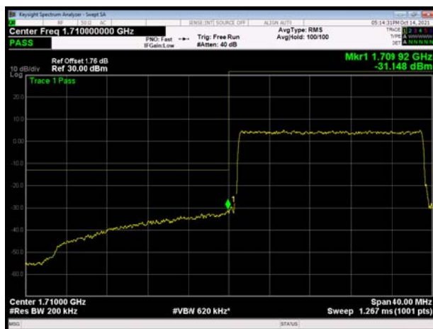
LTE Band 66 QPSK 20MHz CH-Low, 100%RB
