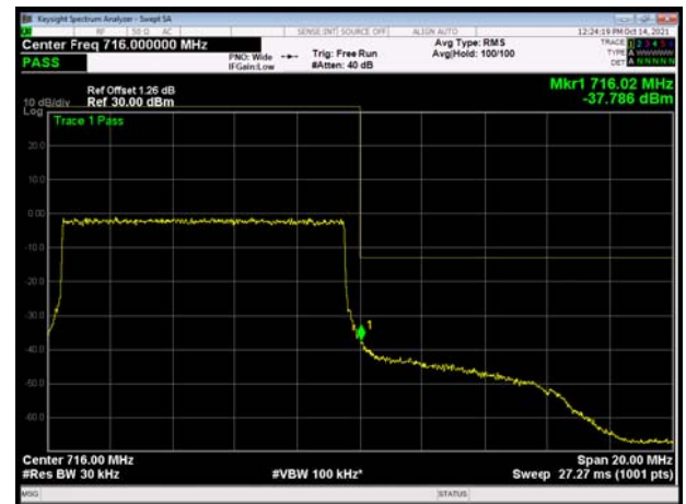
LTE Band 12 64QAM 1.4MHz CH-High, 1 RB
