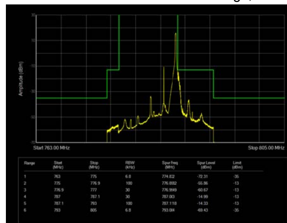
LTE Band 13 16QAM 5MHz CH-High, 100%RB
