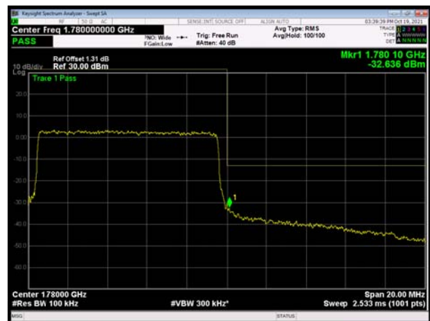
LTE Band 66 64QAM 15MHz CH-High, 1 RB
