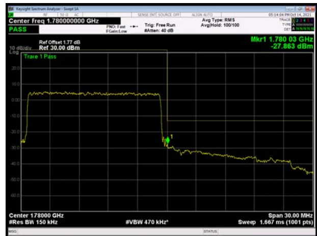
LTE Band 66 QPSK 20MHz CH-High, 1 RB
