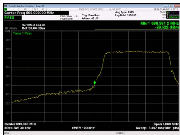
LTE Band 12 64QAM 1.4MHz CH-Low, 100%RB
