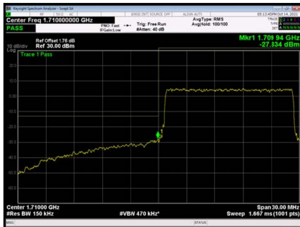
LTE Band 66 QPSK 20MHz CH-Low, 1 RB
