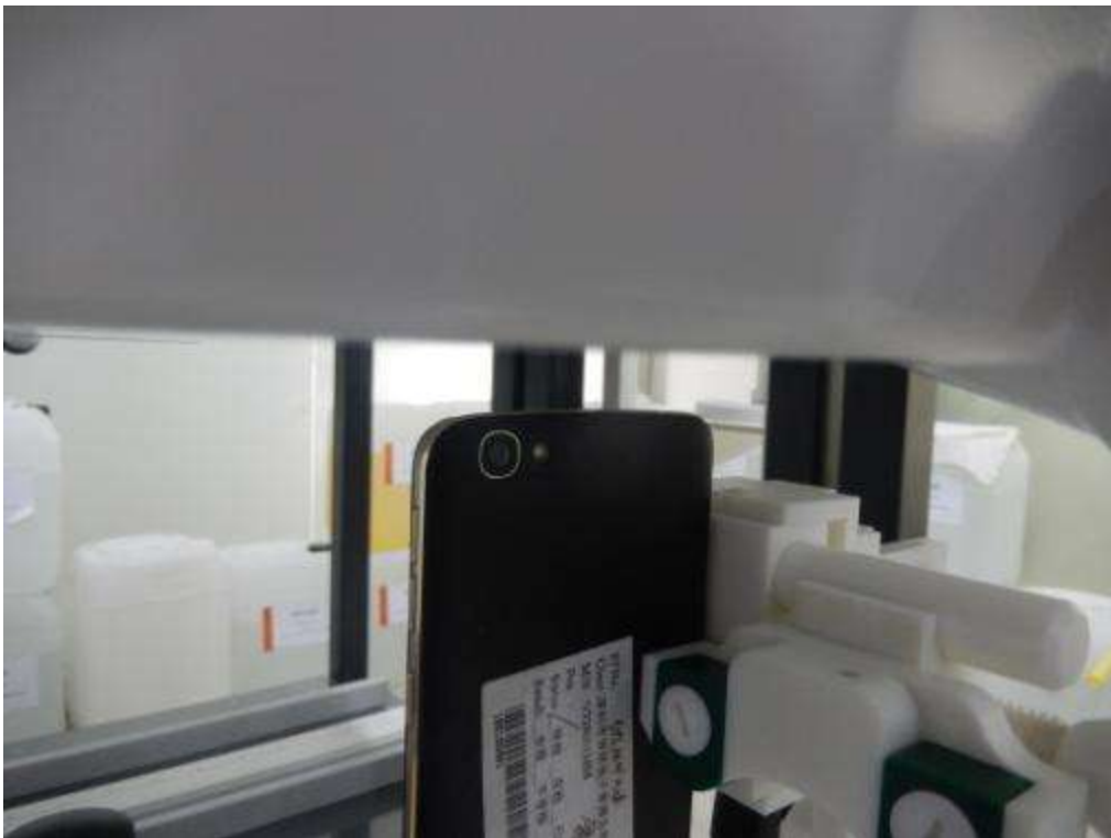
Body Top side (separation distance is 10mm)
