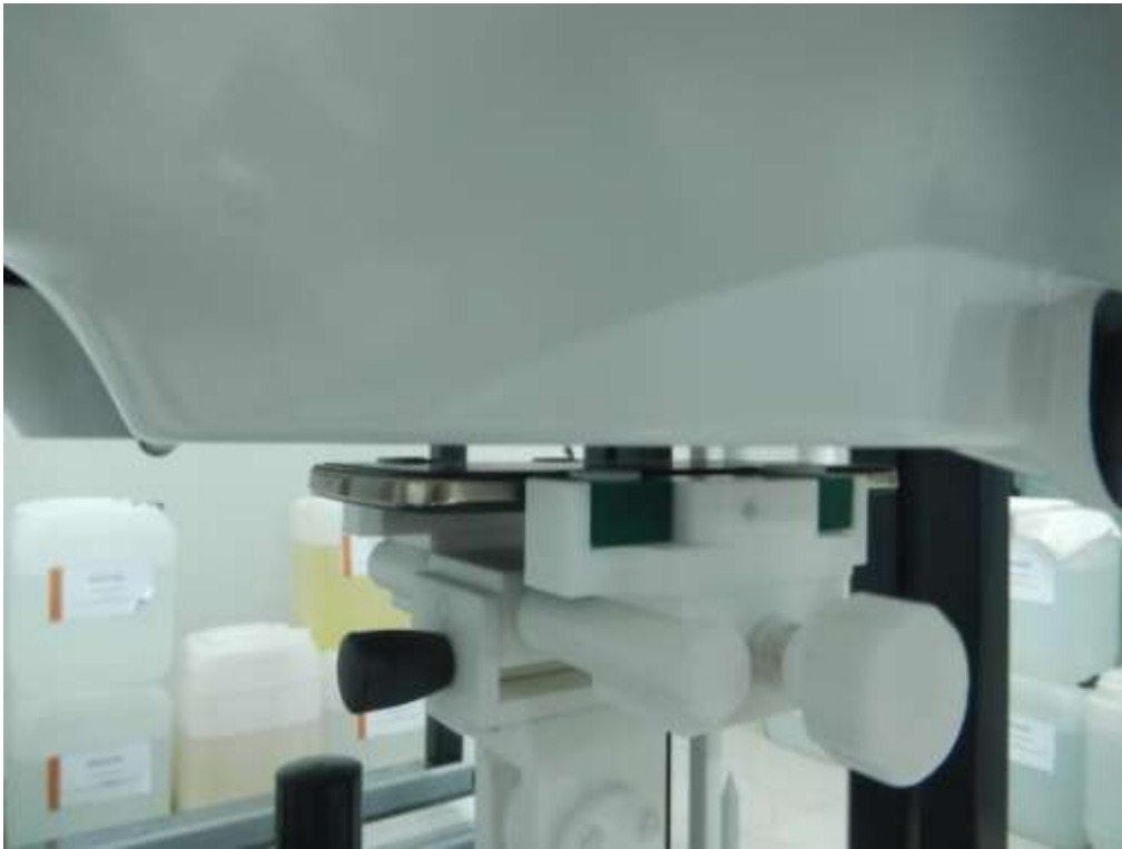
Body Front side (separation distance is 5mm)
